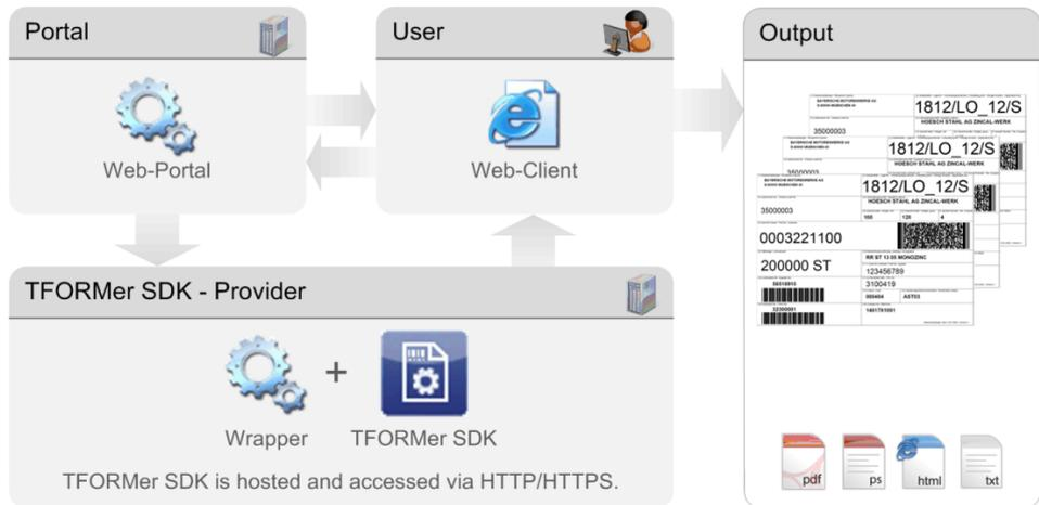
Output creation is triggered with http/https requests. Such requests are integrated easily into each web-application or web-portal (GET/POST requests). The generated output is made available for download, emailed directly to the client or displayed within the client's browser by setting the appropriate MIME type.
